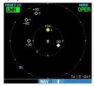
The name of the selected altitude display mode (ABV: look up, NRM: normal, BLW: look down, or UNR: unrestricted) is displayed in the upper left-hand corner of the Traffic Screen. The SKY 497 continues to track up to 30 intruder aircraft within its maximum surveillance range, regardless of the altitude display mode selected.
