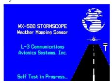
The 400W/500W Series units perform a selftest during power-up to ensure proper operation of the applicable interface components.
