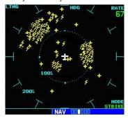
For lightning display interpretation, study the examples in the WX-500 Pilot's Guide that are designed to help you relate the cell or strike patterns shown on the display to the size and location of thunderstorms that may be near your aircraft.
