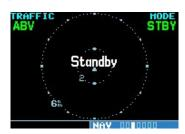
The Standby Screen appears when the SKYWATCH passes the power-up test. NOTE: when the system is in standby, the SKY-WATCH does not transmit, interrogate, or track intruders aircraft.
