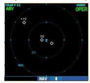
Traffic Page showing Bendix/King KTA 870/ KMH traffic near the 40 nautical mile range, at 10 o'clock above.
